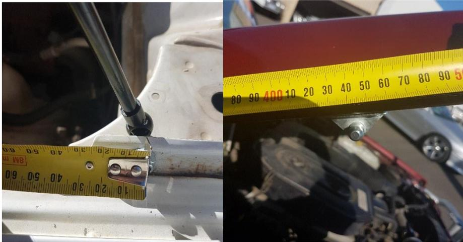
3. Put the strut on bottom ball and bring it up with bracket and mark where to mount. There is enough stroke on the strut to allow the bonnet to lift higher by approx. 100mm. Use a stick etc to hold bonnet higher if you wish, then mark it. You may have to trim back the sound insulation. Mount brackets with nutserts as shown. Keep the strut as square as possible.
